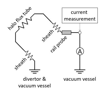
$$V_{\text{halo}} = I_{\text{measured}} \times \mathbf{R_{halo}} + V_{\text{measured}}$$
