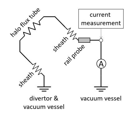
$$V_{\text{halo}} = I_{\text{measured}} \times \mathbf{R_{halo}} + V_{\text{measured}}$$
