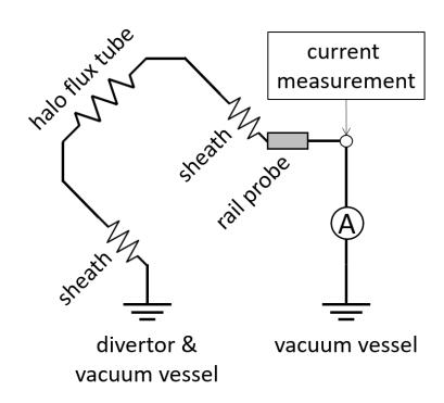
$$V_{\text{halo}} = I_{\text{measured}} \times \mathbf{R_{halo}} + V_{\text{measured}}$$
